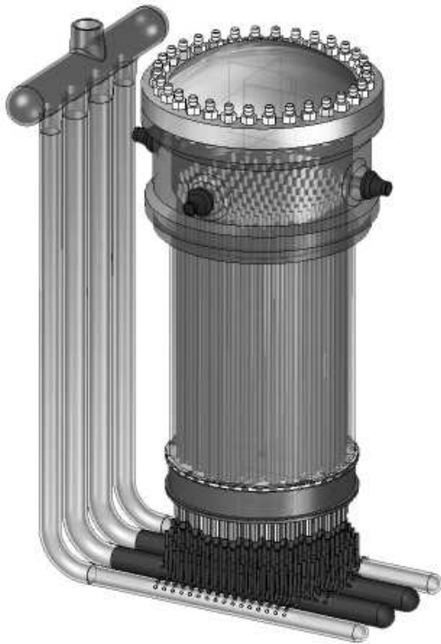
Figure 6. Vertical core-configuration option (courtesy of AECL)
