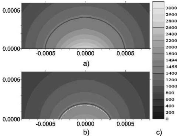
**Fig. 5.** Temperature distribution in samples, made of powders PGSR-3 and PG-10K-01 ( $P_m=150$  W,  $r_p=0,4$  mm,  $V_x=2$  mm/s, air contents – 5%) where:
