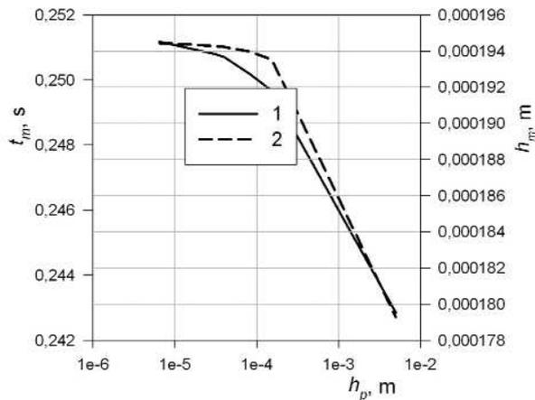
**Fig. 6.** Parameters of a melt pool (depth  $h_m$ , time of existence  $t_m$ ) in a sample made of composition of powder PGSR-3 and an alloyed powder PGSR-3 to thickness of the powder layer  $h_p$  ( $P_m=150$  W,  $d_p=0,6$  mm, 10% Air), where:
