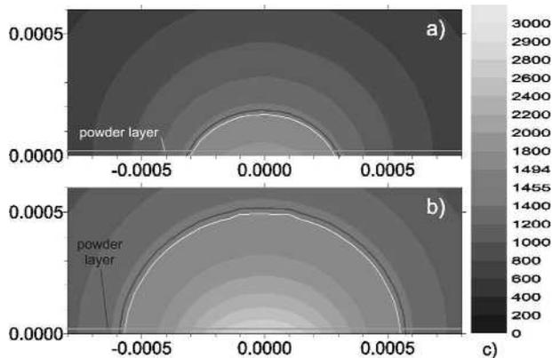
**Fig. 7.** Temperature distribution in a sample made of composition powder PG-10K-01 and an alloyed powder PGSR-3 (a) and in sample made of composition of powder PGSR-3 and an alloyed powder PG 10K-01 (b) ( $P_m = 150$  W,  $r_p = 0,4$  mm,  $V_x = 2$  mm/s, thickness of the powder layer  $h_p = 30$  m and air contents – 10%) where:
