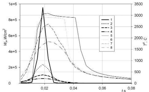
**Fig. 8.** Laser radiation with power density  $W_p(t)$  and surface temperature  $T(0, t)$  of a samples composed of composition powder PGSR-3 and alloyed PGSR-3 powder layer to the size of focusing spot  $r_p$  (thickness of powder layer  $h_p = 30\mu\text{m}$ , 10% Air,  $P_m = 150$  W,  $V_x = 20$  mm/s), where:
