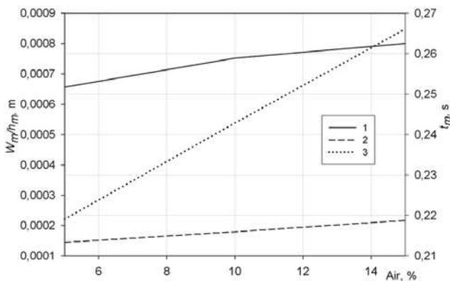
**Fig. 4.** Parameters of a melt pool (width  $W_m$ , depth  $h_m$  and time of existence  $t_m$ ) of sample made of powder PGSR-3 to concentration of an atmosphere (Air, %) ( $P_m=150$  W,  $r_p=0,6$  mm,  $V_x=2$  mm/s), where:
