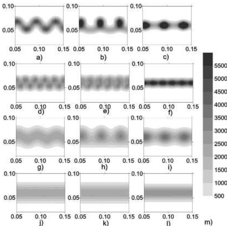
**Fig. 11.** Distribution of energy density  $W_E(x, y)$  in a processing zone ( $P_m = 150 \text{ W}$ ,  $V_x = 20 \text{ mm/s}$ ), with different focused beam sizes and laws of scanning, where:
