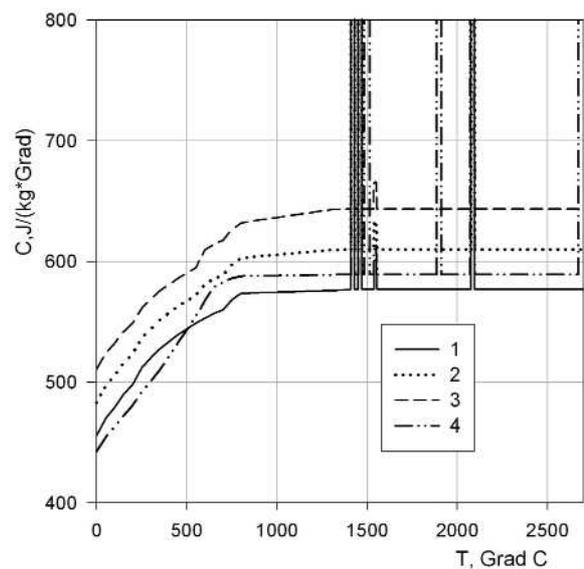
Fig. 3. Heat capacity of material to temperature, where: 1 – alloy on base PGSR-3; 2 – powder PGSR-3 with the contents of an atmosphere of 5%; 3 – powder PGSR-3 with the contents of an atmosphere of 10%;
