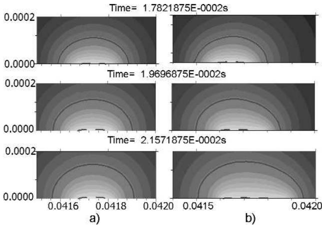
**Fig. 12.** The distribution of temperature in sample for the composition of powder PGSR-3 and alloyed PGSR-3 powder layer ( $P_m = 150$  W,  $r_p = 0.1$  mm,  $V_x = 20$  mm/s, thickness powder layer  $h_p = 30$  μm and air – 10%) where  $a - \omega = 0$  Hz;  $b - A_s = 0$  mm;  $B_s = 0.1$  mm,  $\omega = 100$  Hz; " — " melt pool for Ni; "- - -" vapor pool for Ni
