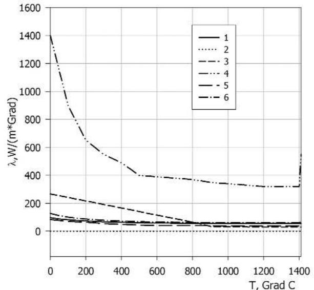
Fig. 2. Heat conductivity of components of powder PGSR-3 and an alloy on a basis of PGSR-3 powder to temperature, where:
