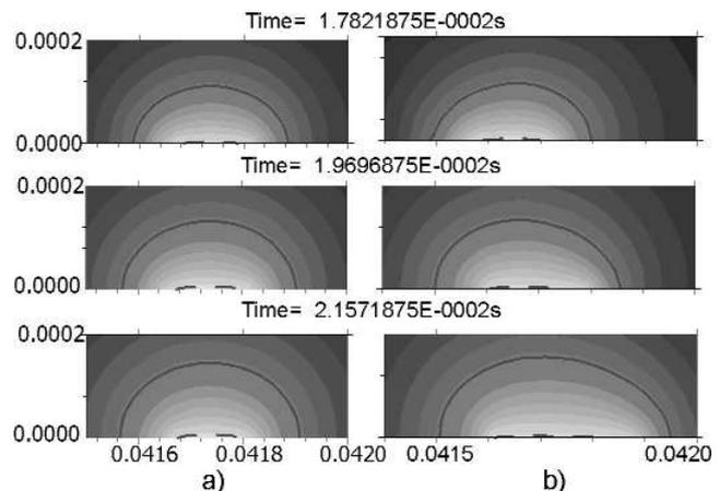
**Fig. 14.** The distribution of temperature in sample for the composition of powder PGSR-3 and alloyed PGSR-3 powder layer ( $P_m = 150$  W, thickness powder layer  $h_p = 30$  μm and air – 10%) where: the size of focusing spot  $r_p = 0.2$  mm  $a - \omega = 0$  Hz;  $b - A_s = 0$  mm;  $B_s = 0.1$  mm,  $\omega = 100$  Hz
