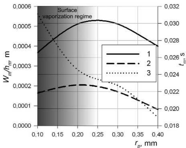
**Fig. 9.** Parameters of a melt pool (depth  $h_m$ , width  $W_m$  and time of existence  $t_m$ ) of a sample composed of the powder PGSR-3 and an alloyed powder layer PGSR-3 to the size of focusing spot  $r_p$  ( $P_m = 150$  W,  $V_x = 20$  mm/s, powder layer thickness  $h_p = 30$  mm, 10% Air) where: 1 – width  $W_m$  of a melt bath to speed  $V_x$ ; 2 – depth  $h_m$  of a melt bath to speed  $V_x$ ; 3 – time of existence  $t_m$  of a melt bath to speed  $V_x$
