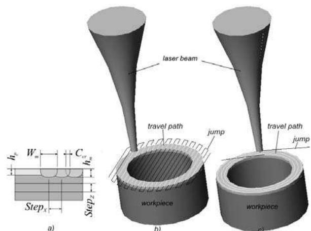
Fig. 1. The scheme of layer dispositions in treated zone, which forms a detail using Rapid Prototyping technology, where:
