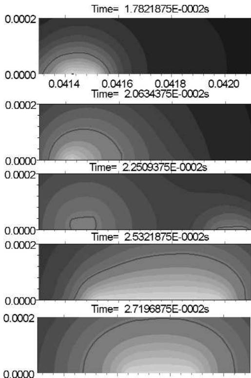
**Fig. 13.** The distribution of temperature in sample for the composition of powder PGSR-3 and alloyed PGSR-3 powder layer ( $P_m = 150$  W,  $r_p = 0.1$  mm,  $V_x = 20$  mm/s, powder layer thickness –  $h_p = 30$  μm and air – 10%,  $A_s = 0.1$  mm;  $B_s = 0.3$  mm,  $\omega = 100$  Hz)
