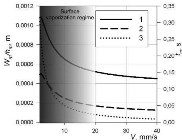
**Fig. 10.** Parameters of a melt pool (depth  $h_m$ , width  $W_m$  and time of existence  $t_m$ ) of a sample composed of powder PGSR-3 and an alloyed PGSR-3 layer powder to processing speed  $V_x$  ( $P_m = 150$  W,  $r_p = 0,3$  mm, thickness of the powder layer  $h_p = 30$  mm, 10% Air): 1 – width  $W_m(V_x)$  of a melt bath to speed  $V_x$ ; 2 – depth  $h_m(V_x)$ ; 3 – time of existence  $t_m(V_x)$
