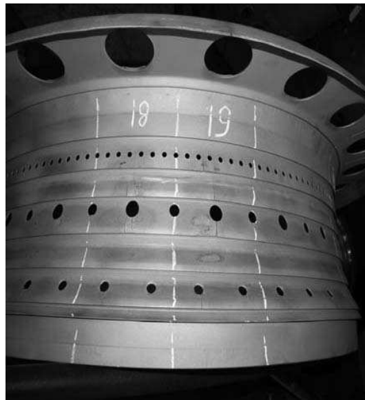
Fig. 3. A combustion chamber internal casing of D-18T engine coated with TZP-3
